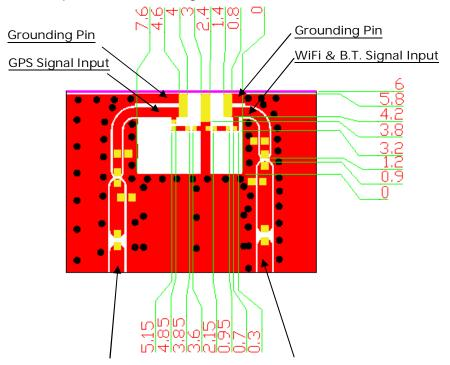
Transmission Line with 50**Ω** Impedance Characteristic
