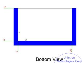
Transmission Line with 50Ω Impedance Characteristic
