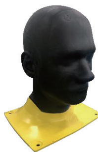
Artificial Head & Artificial Hand for testing wearables and IoT devices
