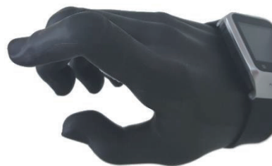
Artificial Head & Artificial Hand for testing wearables and IoT devices
