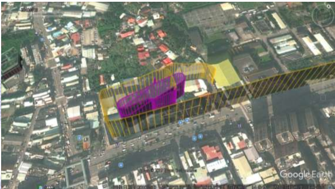
Purple line: underground parking lot
