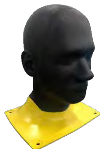
Artificial Head & Artificial Hand for testing wearables and IoT devices
