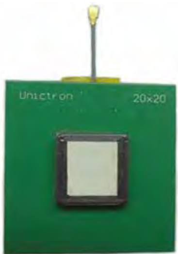
SMD patch antenna 20 × 20 mm on the demo board.
