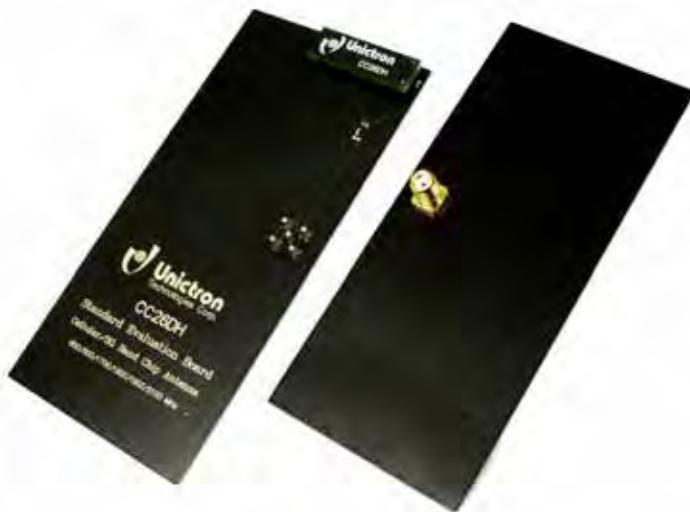
Demo board with GSM chip antenna
